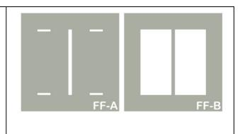
Mask "A" has some additional rectangles cut into the mask which indicate the outer corners of the leading red and trailing blue colours in relation to the white bar.
